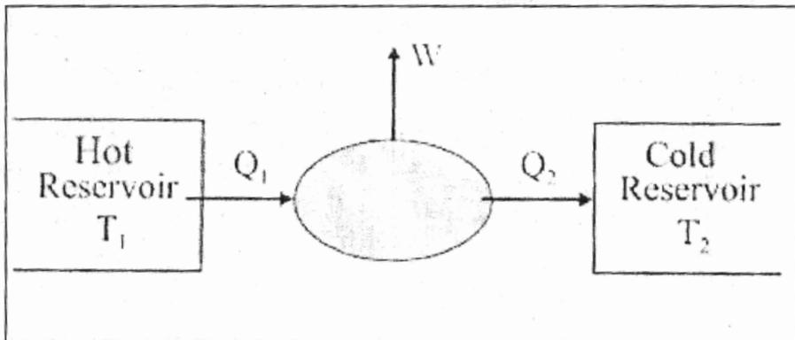
a) Modify the given diagram for a refrigerator. (1)
