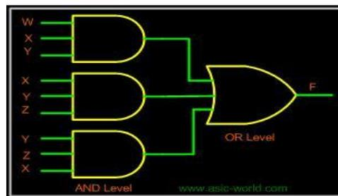
If bubbles are introduced at AND gates output and OR gates inputs (the same for NOR gates), the above circuit becomes as shown in figure
