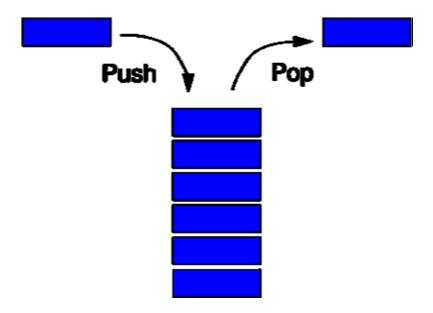
One way to think about this implementation is to think of functions as being stacked on top of each other; the last one added to the stack is the first one taken off. In this way, the data structure itself enforces the proper order of calls.
